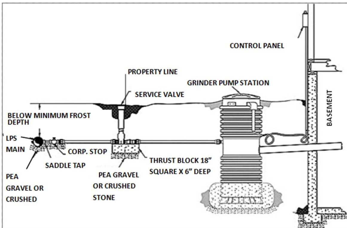
A grinder pump is a pre-fabricated unit that includes a small tank to store wastewater between pump outs. A service valve is installed at the property line to disconnect the service from the LPS system and acts to delineate the private from the public system. A back pressure check valve is installed to avoid sewage from other connected properties flowing back into the grinder pump.
