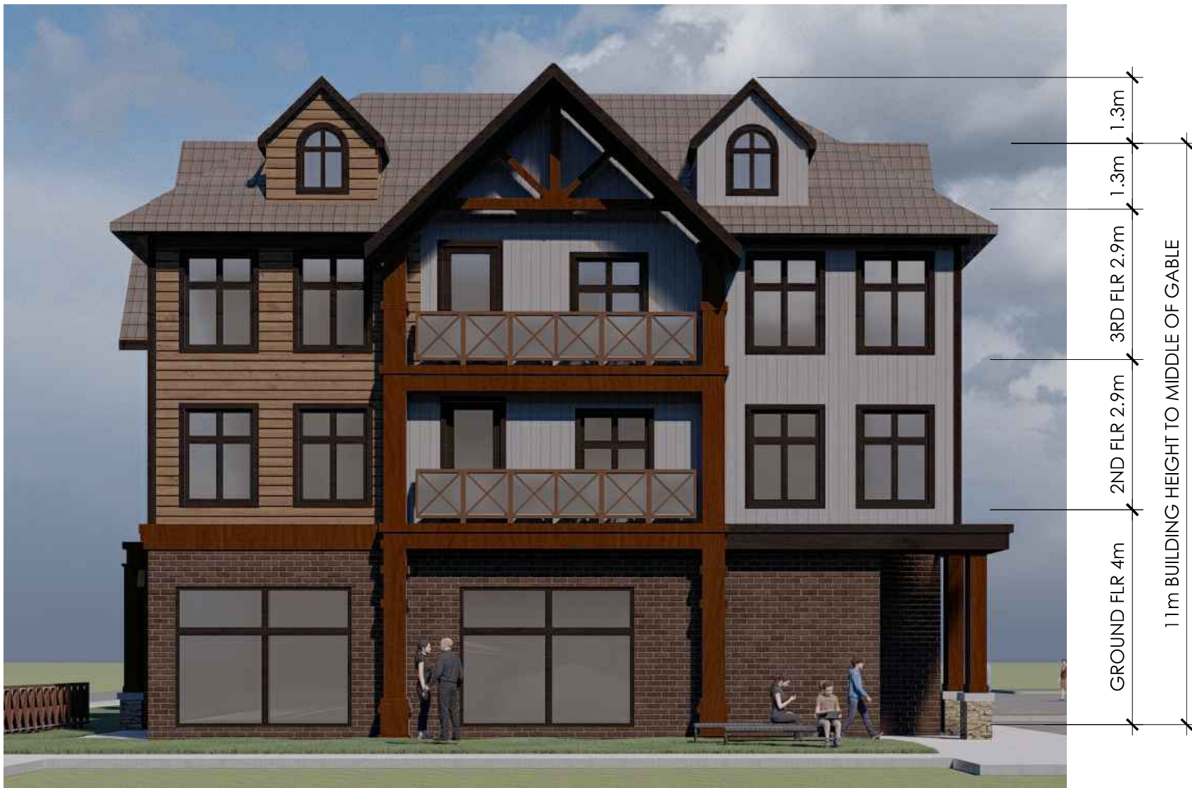
TYP. BUILDING 150 KING ST. - EAST ELEVATION
