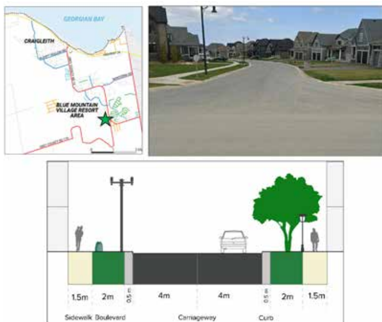
Figure 8-12: Proposed Cross-Section Treatment for Local Roads
