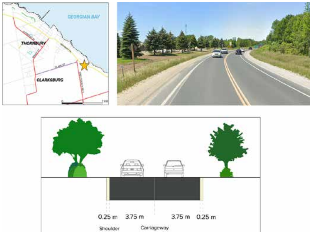
Figure 8-6: Existing Cross Section for Highway 26 (Rural Section)
