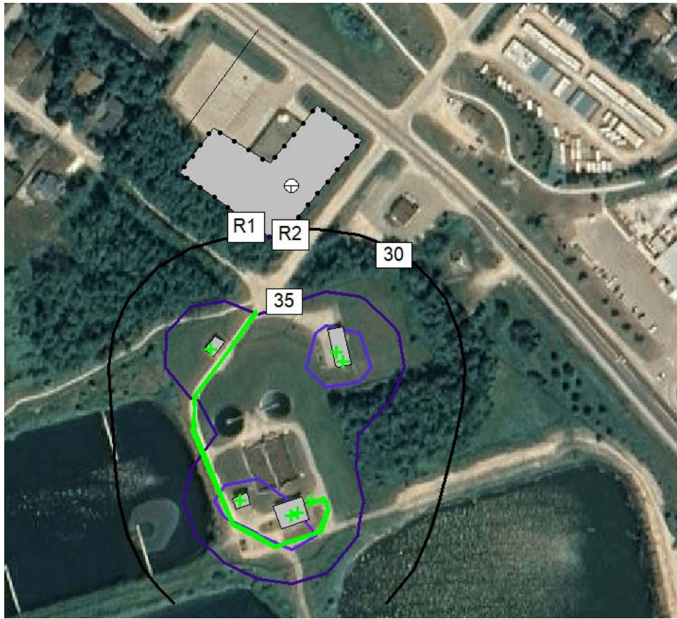
Figure 6: Predicted Night-time Sound Level Contours at 15 m in height
