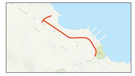
The Town of The Blue Mountains has identified Lakewood Drive for reconstruction due to deficiencies with the water distribution and sewage collection systems. The subdivision was constructed in 1971, and is now due for replacement of the inground works. The road will be reconstructed and the ditches reshaped and cleared of trees.
