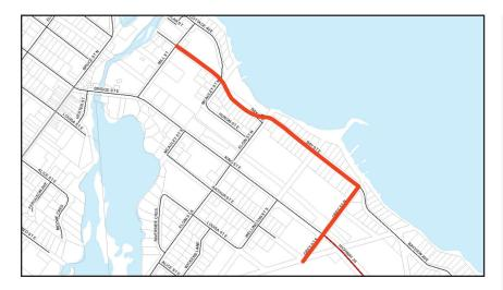
The Town of The Blue Mountains needs to install a secondary sanitary sewer forcemain from the Mill Street Pumping Station to the Thornbury Wastewater Treatment Plant to service growth in the west portion of the municipality. The secondary forcemain will follow Bay Street East between Mill Street and Grey Street, and then proceed south on Grey Street to the treatment plant.
