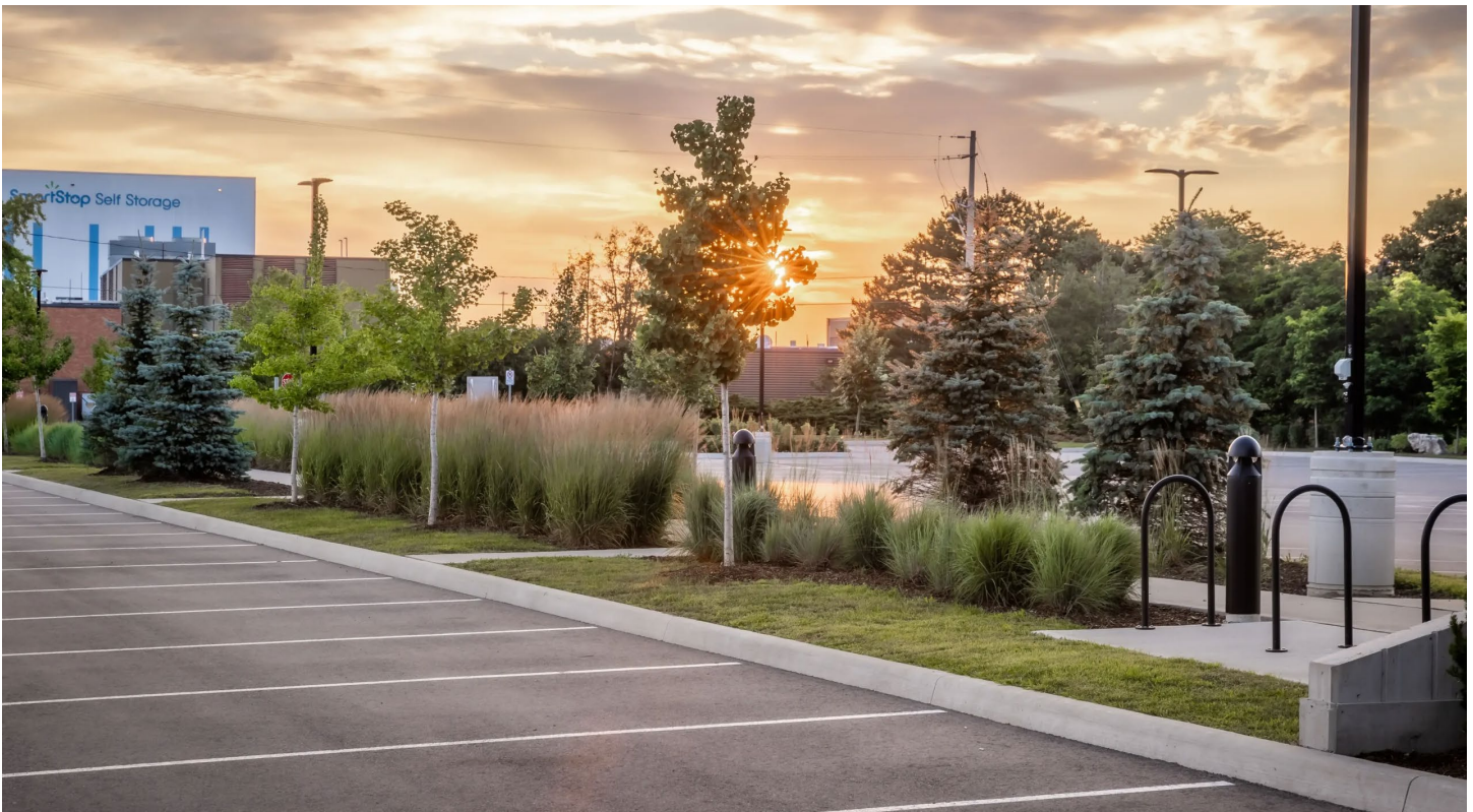
Plant parking islands and walkways to main entrances with a variety of plant materials while also incorporating pedestrian scaled lighting, seating and bicycle racks
