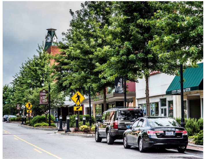
Street parking using a curb extension at the beginning and end
