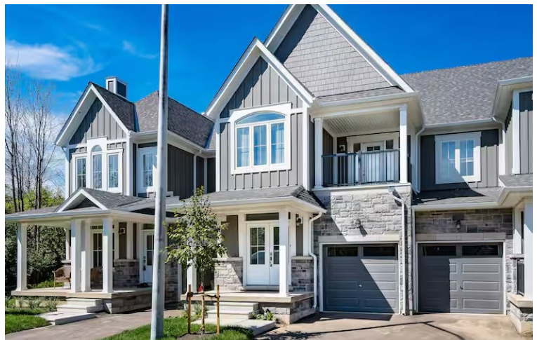
Ensure garages do not project beyond the main wall or in front of a porch and pair driveways where feasible
