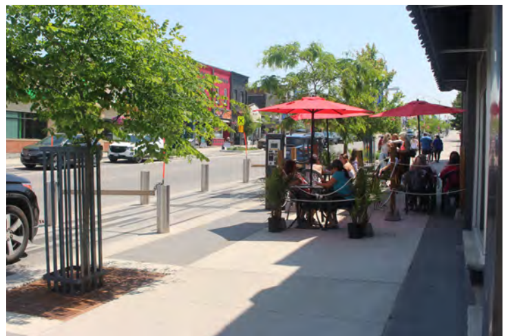
Ensure the alignment of the public sidewalk remains straight within the right-of-way, or alternatively, angled following the configuration of the bump-out along the street
