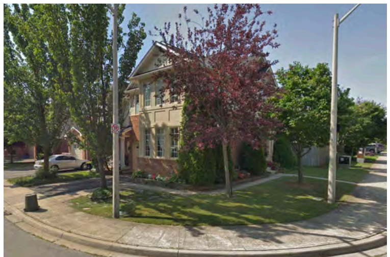
Orient the driveway and garage for corner units to the secondary street and provide the pedestrian entrance from the main street
