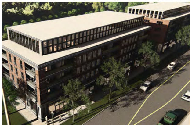
Design taller buildings to incorporate step backs above the second, third or fourth storey
