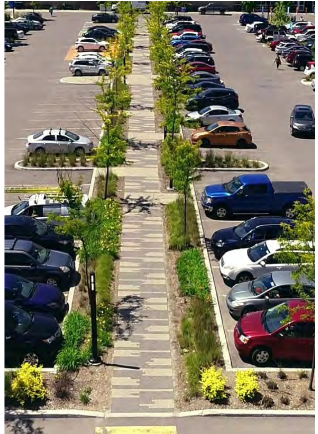
Incorporate a well-defined and continuous pedestrian system with access to the public street, parking and outdoor amenity areas
